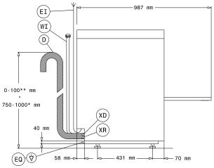
ΕI Electrical inlet (power) EO **Electrical Outlet** HWI Hot water inlet
